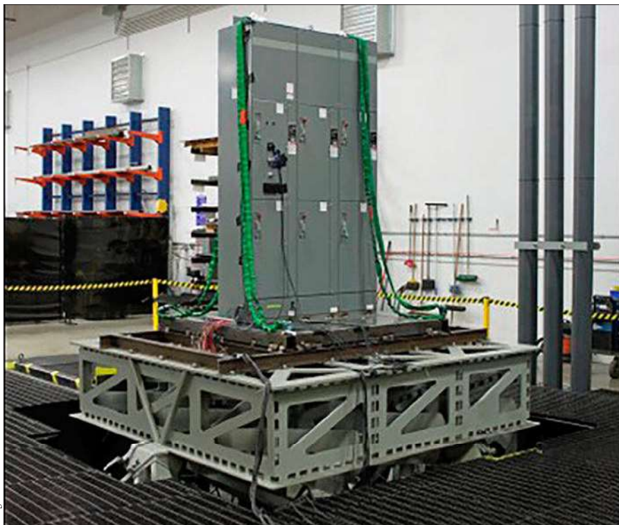
An example of a switch gear panel going through IEEE 344 seismic qualification on a triaxial seismic table.
