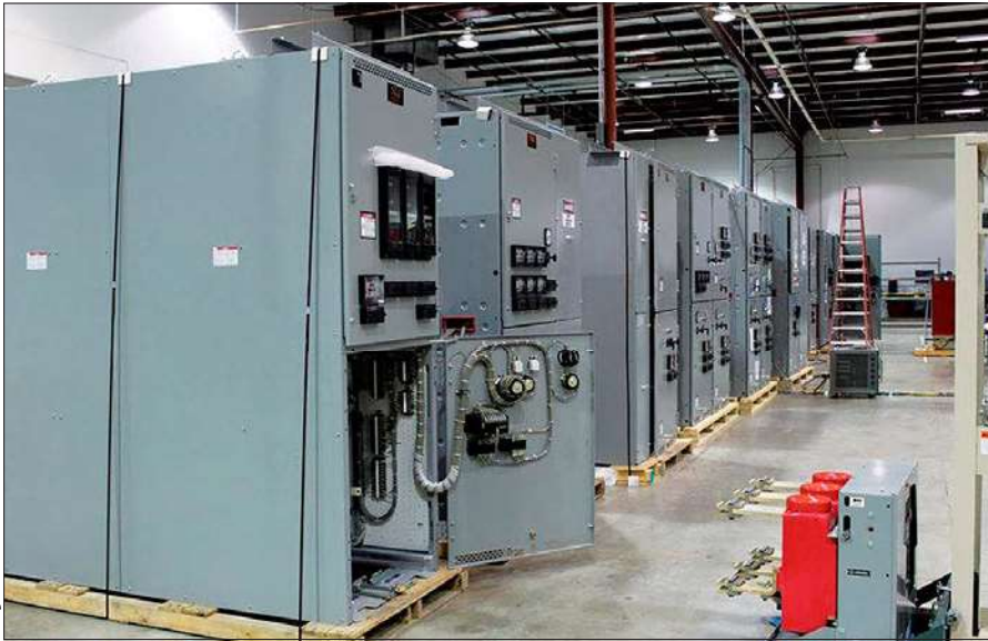
An example of medium voltage switchgear ready to ship to the customer.
